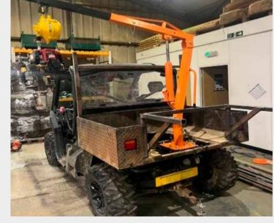
← Photo 3 Operator positioning the post knocker over the post, significantly reducing manual handling
